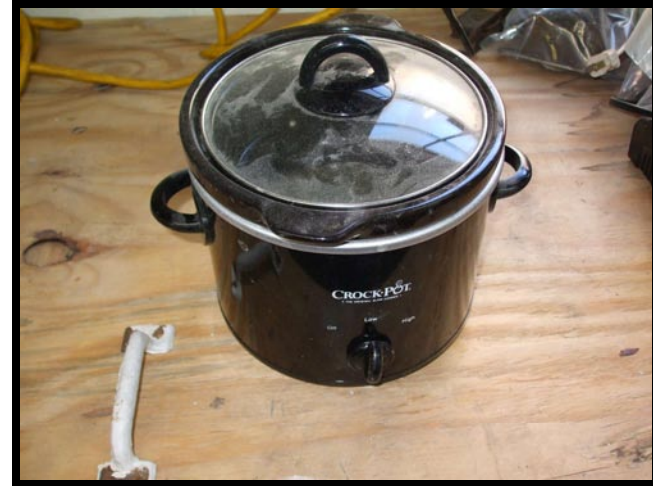
59.) Paint is loosened from hardware with TSP and hot water.
