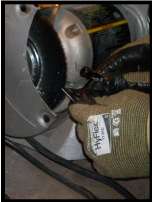
60.) Remaining paint is removed from window latch with a wire wheel.
