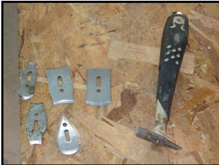
24.) Scraper attachments for paint removal.
